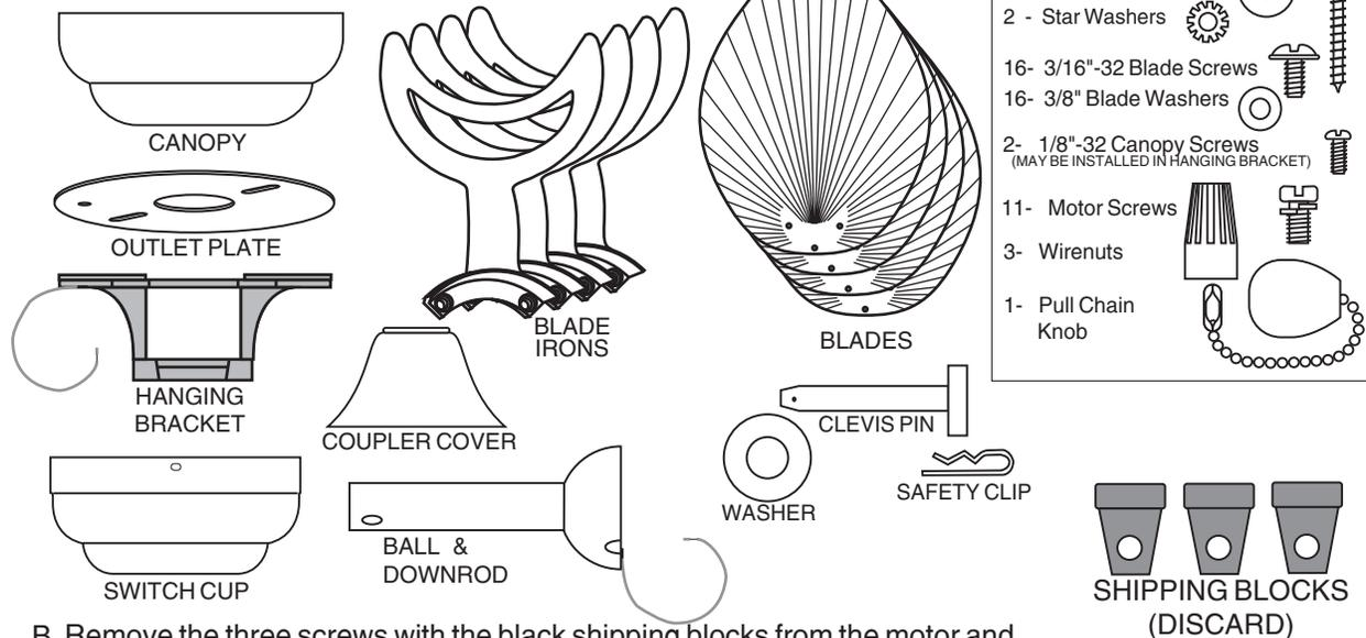
B. Remove the three screws with the black shipping blocks from the motor and discard shipping blocks, if they are present.
